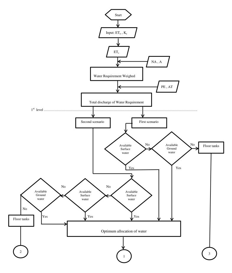
Figure 3: Flowchart illustrates the main steps of mathematical model of conjunctive use.
