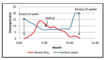
Figure 4: Water requirements discharge with percentage of available surface water 100 %.
