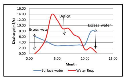
Figure 5: Water requirements discharge with percentage of available surface water 40 % .
