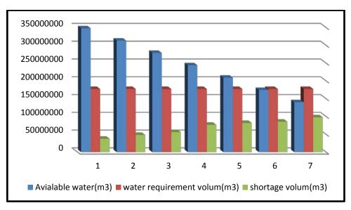
Figure 6: Annual volume of water requirement, available water (surface and ground) and of shortage.
