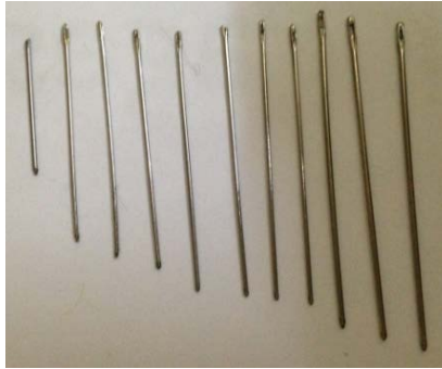
Figure 2: The electrodes used in micro-EDM.
