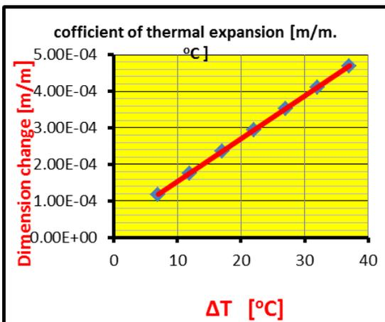
Figure (9): Coefficient of thermal expansion of group (B) materials.
