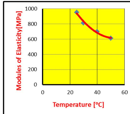
**Figure (12):** Variation of modulus of elasticity with temperature for group (A) of composites column.
