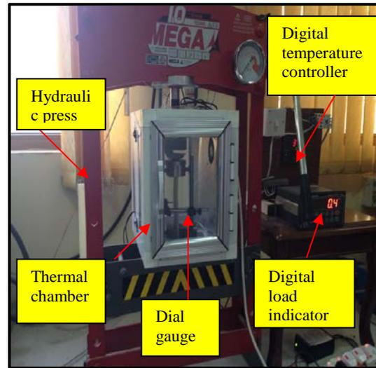
**Figure (3):** Buckling test device
