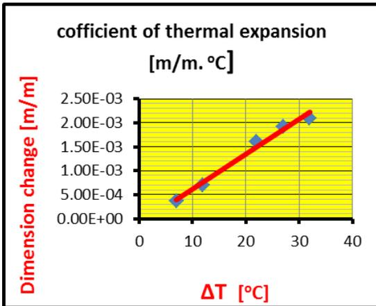
Figure (8): Coefficient of thermal expansion of group (A) materials.
