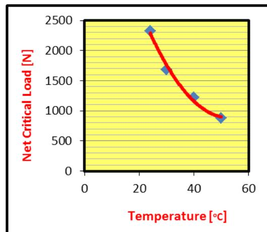
**Figure (11):** Critical buckling load vs. temperature.
