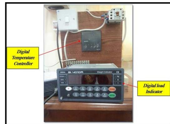
**Figure (5):** Digital load indicator and digital temperature controller
