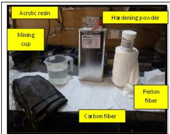
**Figure (1):** The Materials used in the manufacturing of test specimens.
