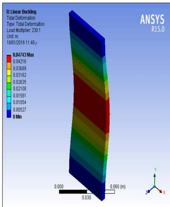
Figure (15): The buckling shape of group (B).
