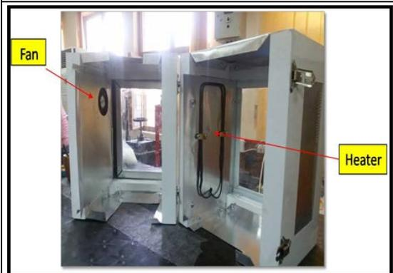
Figure (7): Thermal chamber containing (A) Heater (B) Fan.
