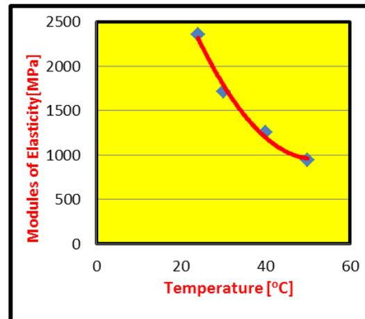
**Figure (13):** Variation of modulus of elasticity with temperature for group (B) of composites column.
