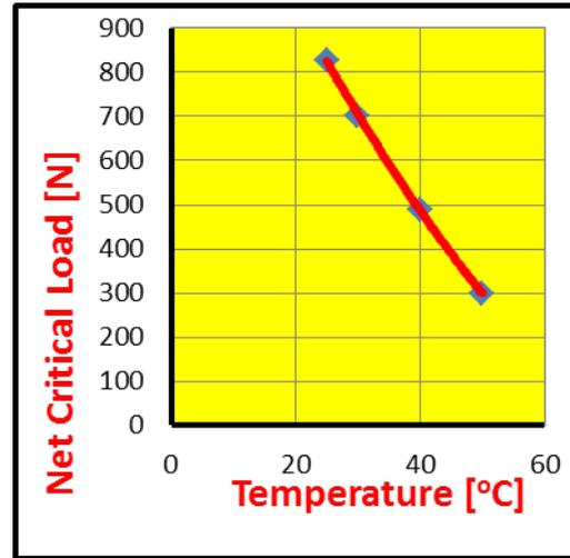
**Figure (10):** Critical buckling load vs. temperature.
