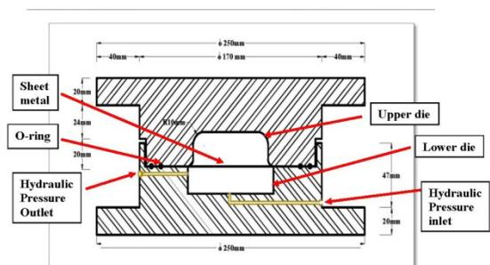
**Figure 4:** First step of the design of the two dies
