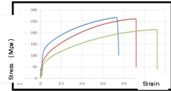
Figure 12: Stress-stain curves for CuZn35, 1.00 mm thick 45° with rolling direction
