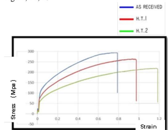
Figure 11: Stress-stain curves for CuZn35, 1.00 mm thick 0° with rolling direction
