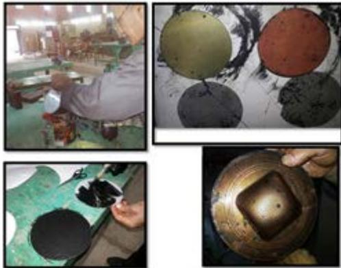
Figure7: Specimen before and after deformation showing the preparation of painting the grid pattern of circles with special metal paint
