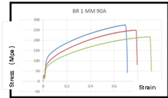
Figure 13: Stress-strain curves for CuZn35, 1.00 mm thick 90° with rolling direction
