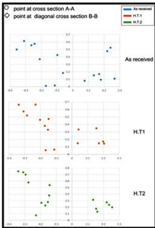
Figure 16 :Strain distribution of CuZn35, 1.0 mm thick
