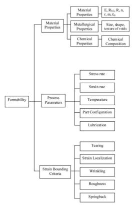
Figure 1: Parameters influencing sheet metal formability [2].
