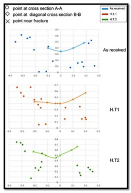
**Figure 17:** Forming limit curve of CuZn35, 1.00 mm thick.
