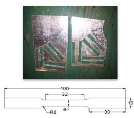
Figure 3: Specimen cut with different rolling directions and standard tensile test dimensions (mm).
