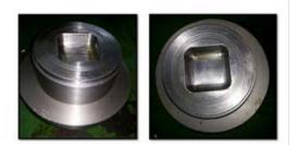
Figure 6 : Final shape of the dies
