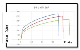
**Figure 13:** Strees-stain curves for CuZn35, 1.00 mm Thick 90° with rolling direction
