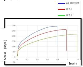
**Figure 11:** Stress-stain curves for CuZn35, 1.00 mm thick 0° with rolling direction
