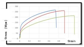
**Figure 12:** Stress-stain curves for CuZn35, 1.00 mm thick 45° with rolling direction
