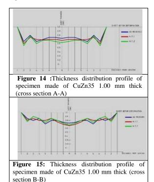
Table 5 shows the percentage of maximum thinning that happened in each specimen for different heat treatment, from which we can see the improvement of maximum thinning for each one by the annealing processes which means decrease in the width which leeds to increase in the strain levels due to annealing process
