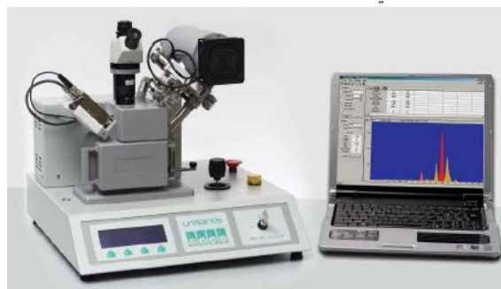
Figure 1: XRF Analyzer (XMF 104) for determine alloying elements percentage.
