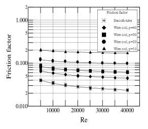
Fig. 5: Friction factor vs. Reynolds number.
