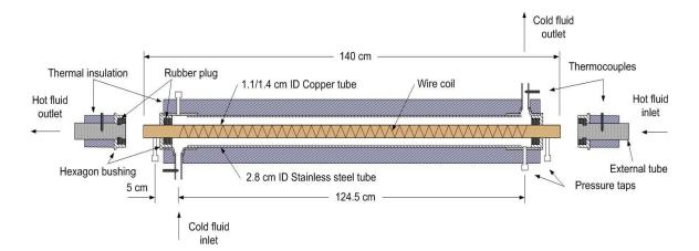
Fig. 2: A sketch of the double pipe heat exchanger
