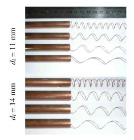
Fig. 3: Wire coils employed in the experiments
