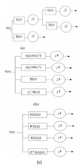
Fig.1 (a) Two-scale iterated filter bank DWT,(b) Equivalent form using DWT,(c) Two-scale filter bank using SLT.
