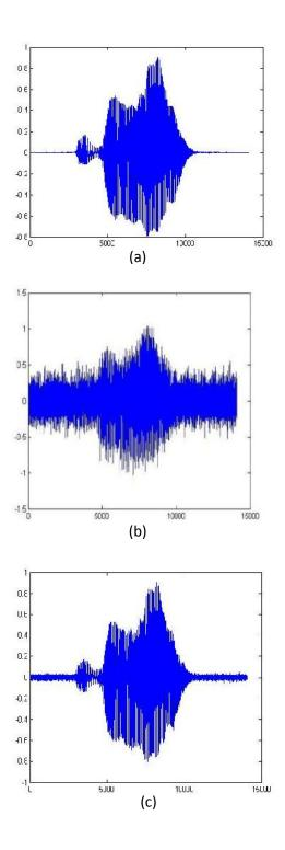
Fig. 4 (a) Clean speech signal,(b) Corrupted signal with noise,(c) Enhanced speech signal
