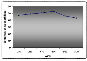
**Figure (4)**: the relationship between the compression strength and weight fraction for polyurethane resin filled with (coconut shell) powders, at a rang of (2-10) % wt.
