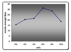
Figure (3) the relationship between the tensile strength and weight fraction for polyurethane resin filled with (coconut shell) powders, at a rang of (2-10) %wt.
