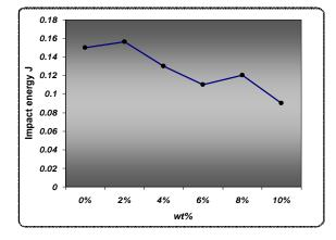
**Figure (5):** the relationship between the impact energy and weight fraction of polyurethane resin filled with (coconut shell) powders, at a range of (2-10) % wt.
