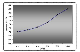
**Figure (6):** the relationship between the hardness and weight fraction for polyurethane resin filled with (coconut shell) powders, at a rang of (2-10) % wt.
