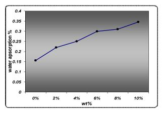
**Figure (7):** the relationship between the water absorption percentage and weight fraction for polyurethane resin filled with (coconut shell) powders, at a rang of (2-10) % wt.
