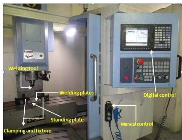
Figure 3: Schematic of friction stir welding (FSW) for plates
