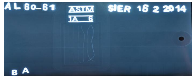
Figure 20: X-Ray Radiographic for FSP of 6061-T6AA at 1300 rpm, 60 mm/min.
