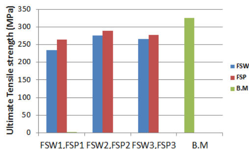
Figure 16: Ultimate Strength Results Results for 6061-T6
