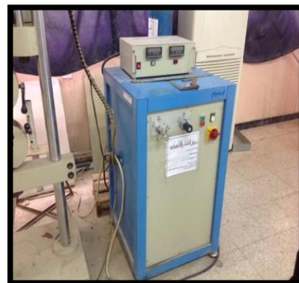
**Figure 7:** Tension Machine for flat specimen
