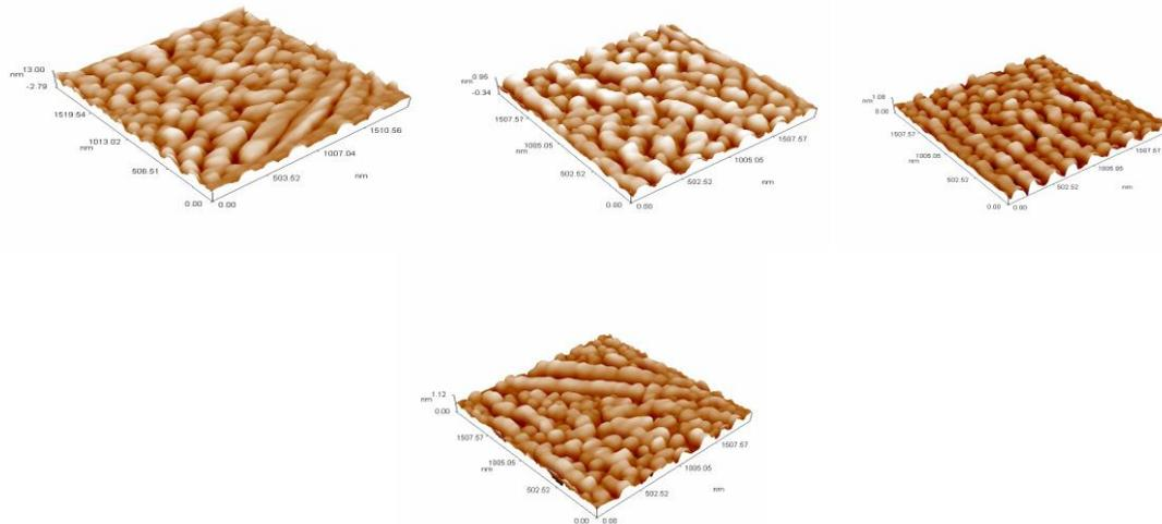
**Figure 19:** Atomic force microscopy of epoxy, aluminum, titanium dioxide and zinc respectively.
