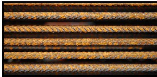
**Figure 1:** Corrosion of steel bar [2]
