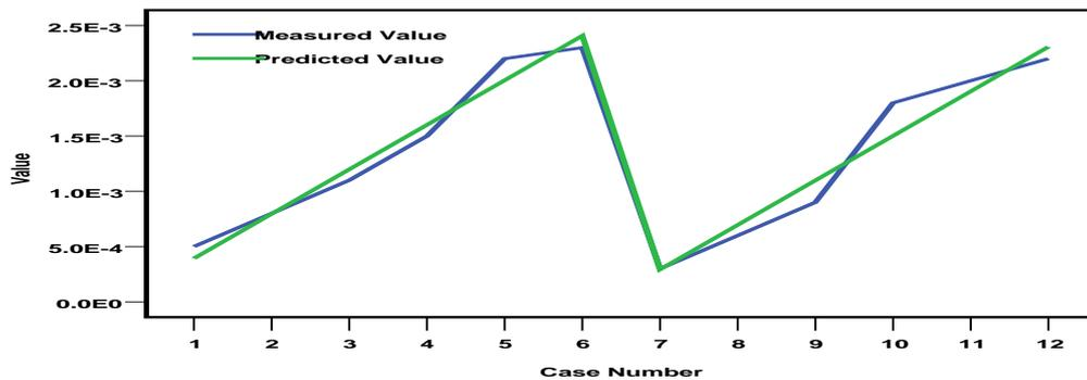
Figure 17: Comparison between measured and predicted values for the experimental data of erosion rate for 100%Epoxy spray pyrolysis (caseA<sub>4</sub>)
