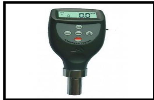
**Figure 6:** Durometer Hardness instrument of type (Shore D).
