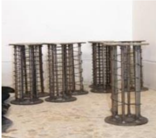
Figure 2: The internal reinforcement is samples with end bracing
