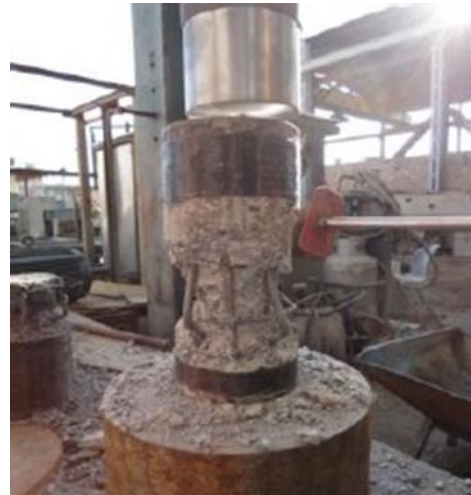
Figure 11: Final failure due to the yield effect and buckling of longitudinal steel bars and sheet failure
