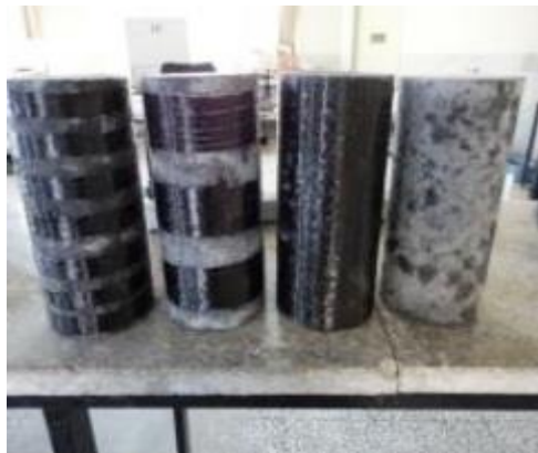
Figure 3: The external reinforcement in the experimental samples
