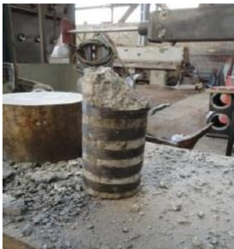
Figure 10: CFRP sheet failure and sample collapse
