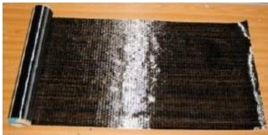
Figure 4: Carbon fibers used in this research
