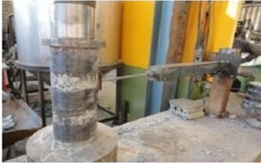
Figure 6: Loading and recording the longitudinal and transverse strains in the samples
