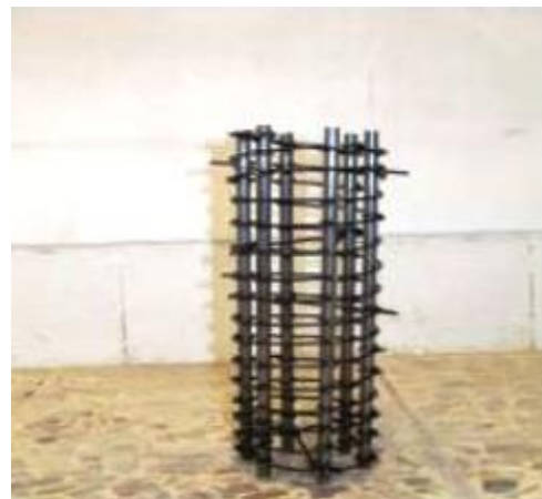
Figure 1: The internal reinforcement in samples without end bracing
