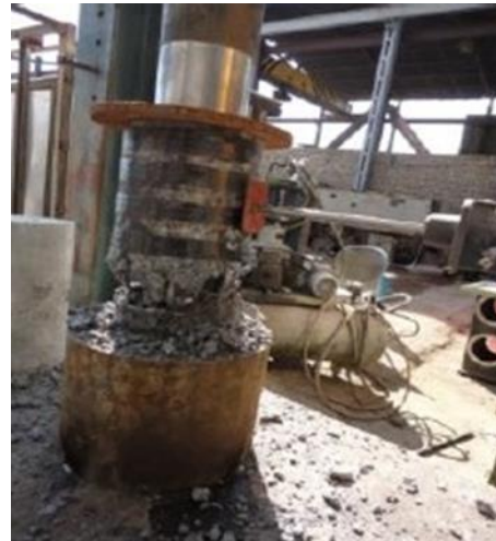
Figure 12: Final failure due to the yield effect and buckling of longitudinal steel bars and sheet failure
