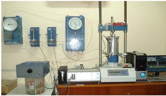
**Figure 5:** Photograph of the suction-controlled triaxial equipment
