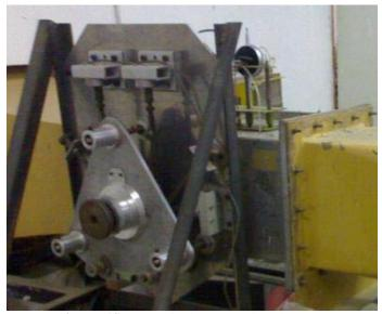
Figure (4): Electrical three weight balance
