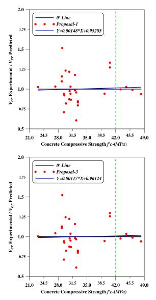
**Figure 4:** Concrete Compressive Strength *f*'*c* versus Ratio of Experimental to Predicted Cracking Shear Strengths-*V*<sub>cr</sub>
