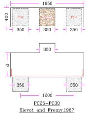
**Figure 1:** Pile Caps Geometry and Section for Use in Statistical Analysis
