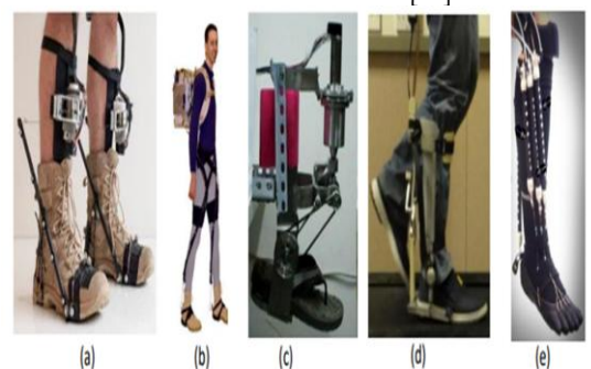
Figure (6): One-DoF ankle exoskeleton (a) [41]; (b) [42]; (c) [43]; (d) [44]; and (e) [45]
