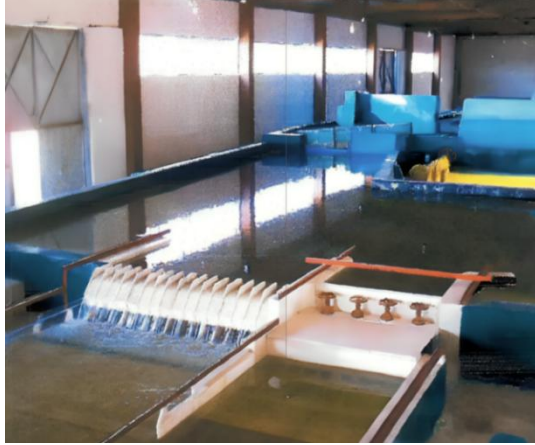
Figure 2: The physical model of dam structures
