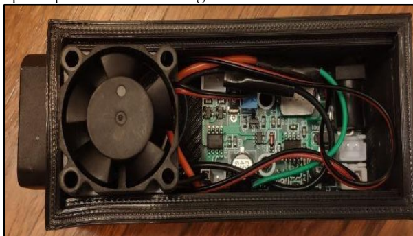
Figure (5): White laser with cooling fan.
