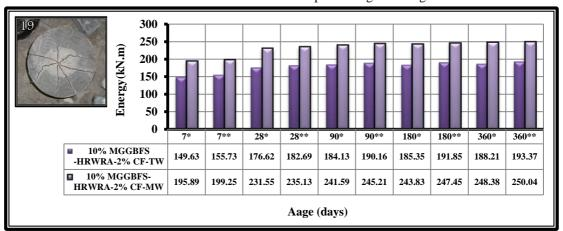
Figure 18: Effect of magnetic mixtures containing 10% MGGBFS- HRWRA reinforced with micro carbon fibers on the impact strength with age.
