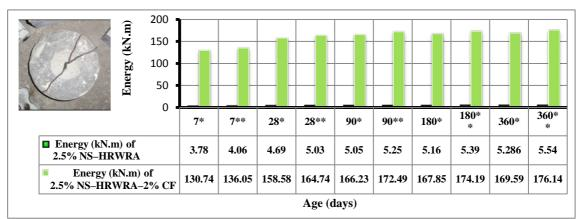
Figure 9: Effect of nonmagnetic mixtures containing 2.5% NS-HRWRA reinforced with micro carbon fibers on the impact strength with age.
