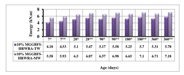
Figure 15: Effect of magnetic mixtures containing 10% MGGBFS-HRWRA on the impact strength with age.
