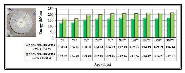
Figure 16: Effect of magnetic mixtures containing 2.5% NS-HRWRA reinforced with micro carbon fibers on the impact strength with age.
