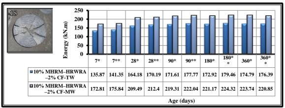
Figure 17: Effect of magnetic mixtures containing 10%MHRM-HRWRA reinforced with micro carbon fibers on the impact strength with age.
