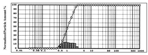
Particle Diameter (μm) Figure 3: Particle size distributions of Micro Ground Granulated Blast-Furnace Slag MGGBFS)
