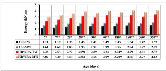
Figure12: Effect of magnetic mixture of CC containing HRWRA on the impact strength with age.
