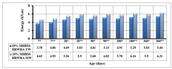
Figure 14: Effect of magnetic mixtures containing 10% MHRM-HRWRA on the impact strength with age.
