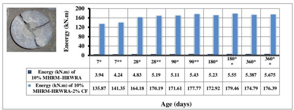
Figure 10: Effect of nonmagnetic mixtures containing 10% MHRM-HRWRA reinforced with micro carbon fibers on the impact strength with age.
