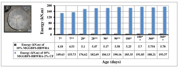
Figure 11: Effect of nonmagnetic mixtures containing 10% MGGBFS-HRWRA reinforced with micro carbon fibers on the impact strength with age
