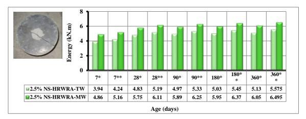
Figure 13: Effect of magnetic mixtures containing 2.5% NS-HRWRA on the impact strength with age.
