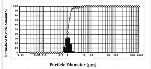
Figure 5: Particle size distributions of metakaolin
