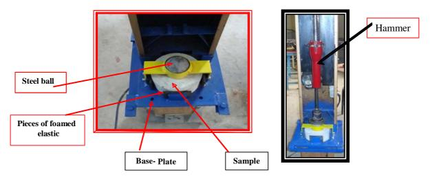
Figure 6: The arrangement of the impact equipment for measurement impact strength
