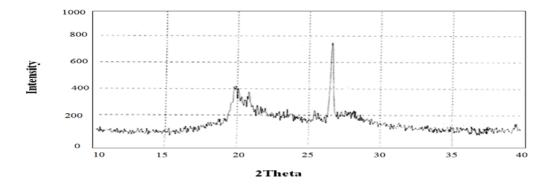
**Figure 4:** X-Ray diffraction patterns of Kaolinite clay calcined at 700<sup>O</sup> C for one hour then rapidly quenching in water
