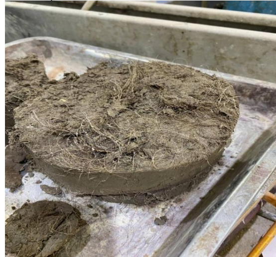
Figure (18): Soil sample mixed with HHF cut in half after CBR test performed.
