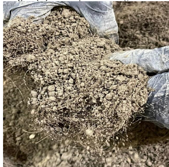
Figure (13): Close up photo of the mixed soil sample with HHF.
