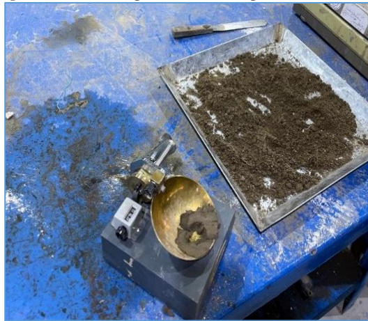
Figure (5): Casagrande Device.
