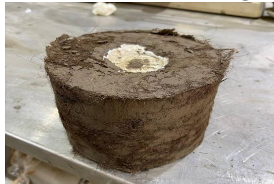
Figure (17): Soil sample mixed with HHF after CBR test performed and extracted from the mold.
