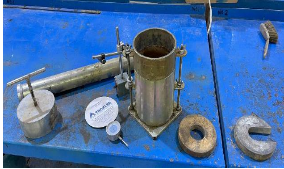
Figure (14): CBR standard mold.
