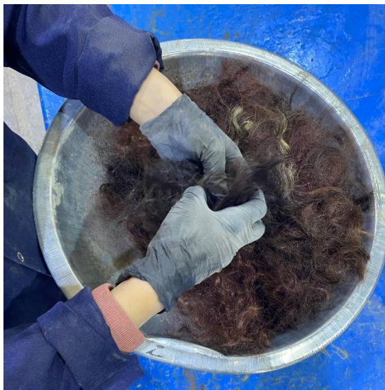
Figure (10): Prepare the human hair by separating the strands to enhance mixing with the soil.
