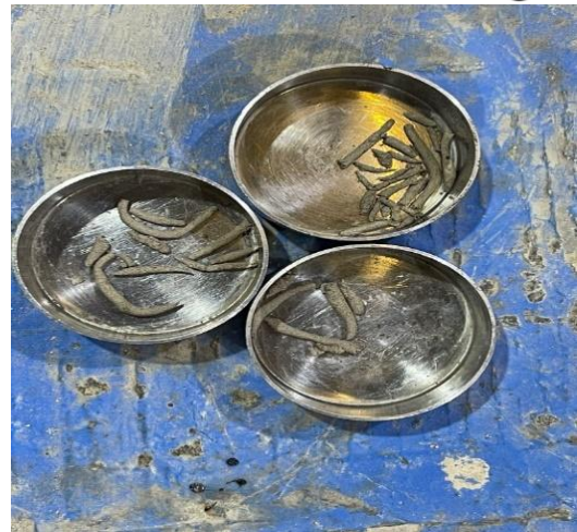
Figure (7): The plastic limit samples.
