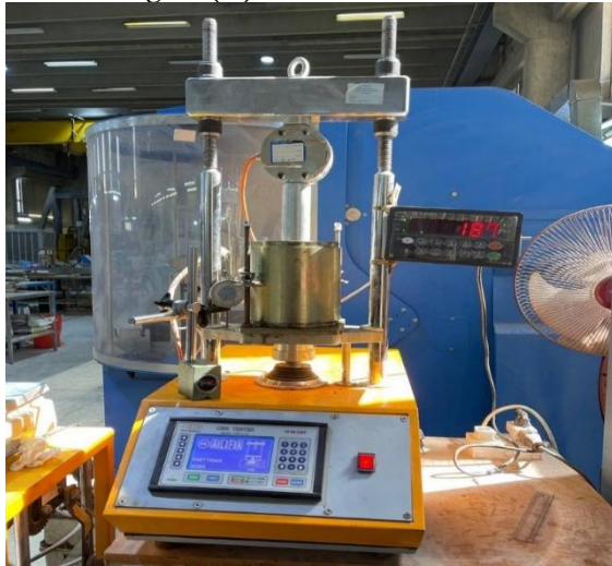
Figure (15): CBR tester machine.
