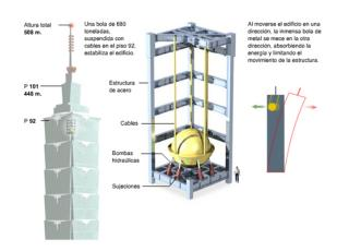
Figure10: Taipei 101 Tower's TMD system. source [14]
