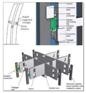
**Figure 6:** Example of a viscous dampers system applied to a Diagrid structure source[7]
