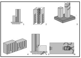
**Figure 3:** the systems configuration of tall building that should be avoided in seismic design [17] p.29-31
