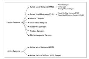
Figure 7: Auxiliary damping systems for tall buildings, source [19]
