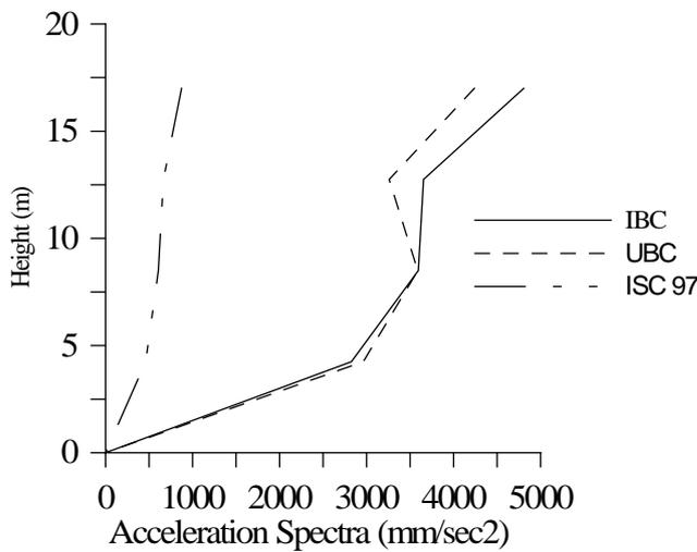
**Figure 11:** Comparison of Story Scaled Acceleration Spectra for EQ in X-direction.
