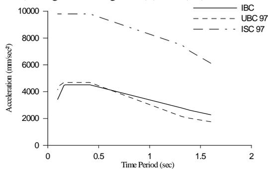
Figure 9: Comparison of Response Spectrum Modal in X-Direction for 5% Damping.
