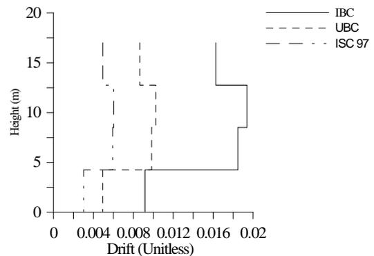
**Figure 7:** Comparison of Maximum Story Drift for EQ in X-direction.
