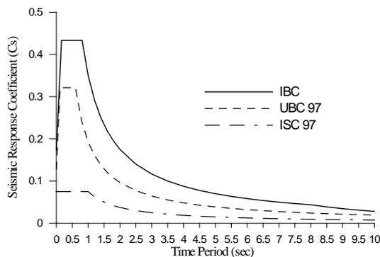
**Figure 3:** Comparison of Seismic Response Coefficient.
