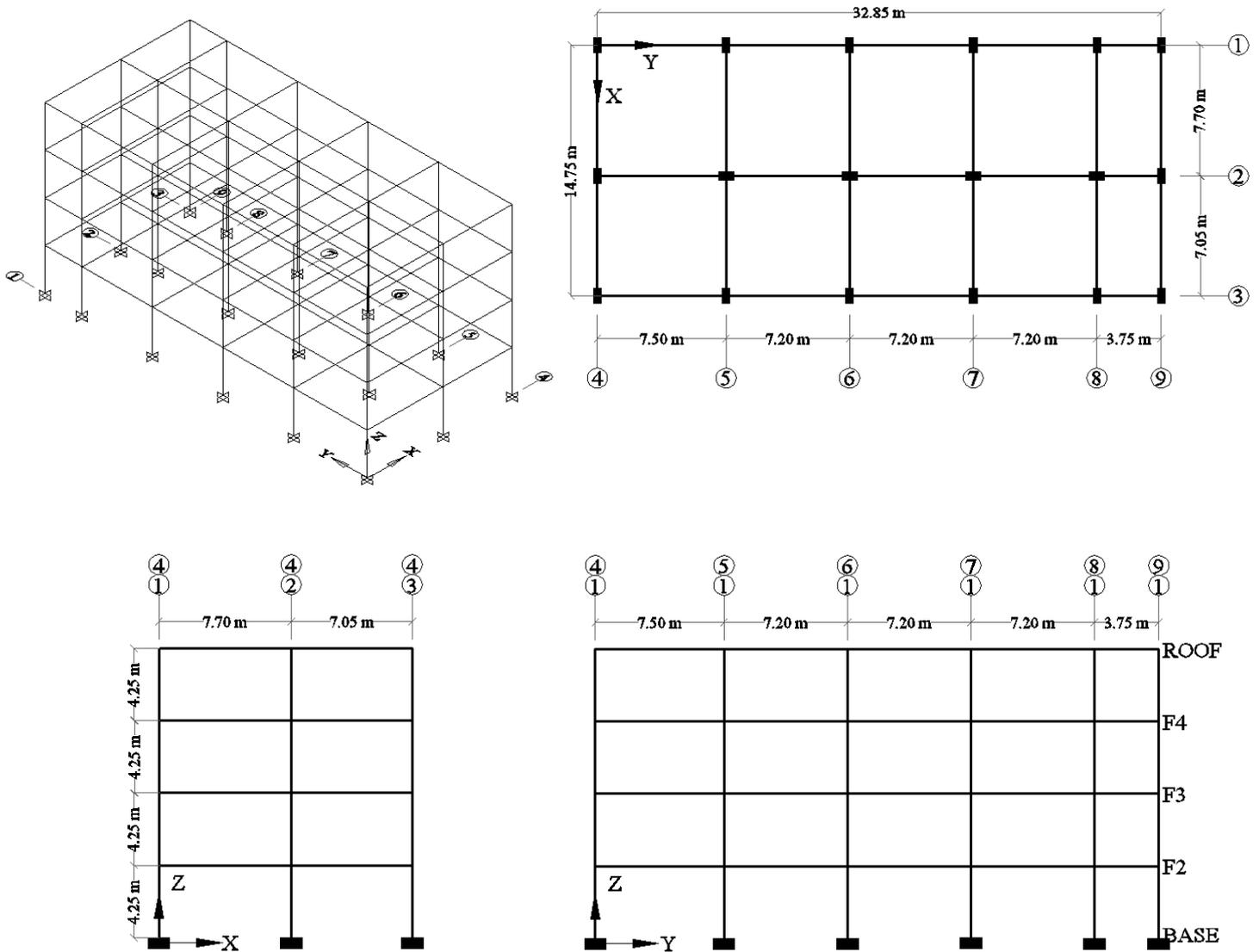
Figure 1: Three-Dimensional Computer Model and Geometry of the Building.
