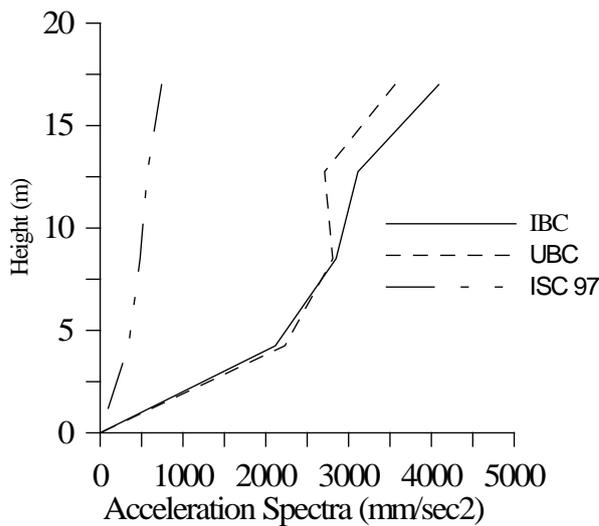
**Figure 12:** Comparison of Story Scaled Acceleration Spectra for EQ in Y-direction.
