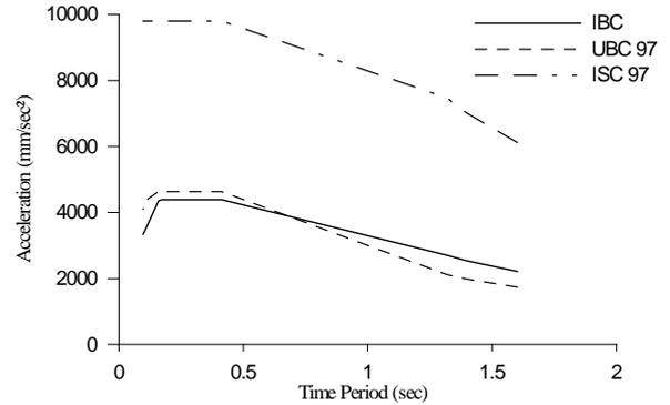
Figure 10: Comparison of Response Spectrum Modal in Y-Direction for 5% Damping.
