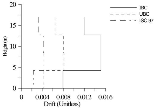
Figure 8: Comparison of Maximum Story Drift for EQ in Y- direction.
