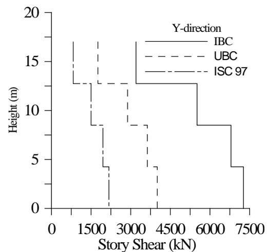
**Figure 13:** Comparison of Story Shears for EQ in X and Y-directions respectively
