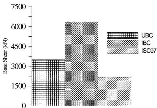
**Figure 5:** Comparison of Base Shears Defined in the Codes for EQ in X-direction.
