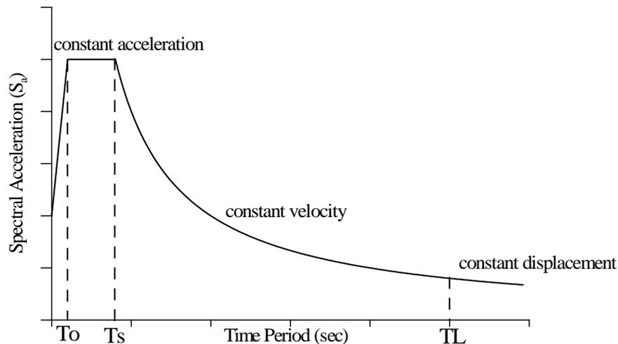
Figure 2: Typical Horizontal Elastic Design Spectrum.
