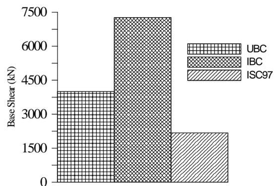
**Figure 6:** Comparison of Base Shears Defined in the Codes for EQ in Y-direction.
