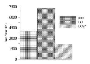
Figure 6: Comparison of Base Shears Defined in the Codes for EQ in Y-direction.
