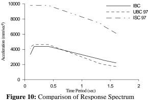
Figure 10: Comparison of Response Spectrum Modal in Y-Direction for 5% Damping.
