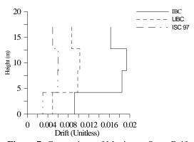
Figure 7: Comparison of Maximum Story Drift for EQ in X –direction.
