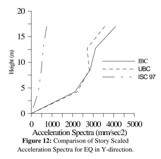
The analysis results show that the computed maximum floor acceleration of IBC is increased by (13%) and decreased by (13%) compared with maximum computed floor
