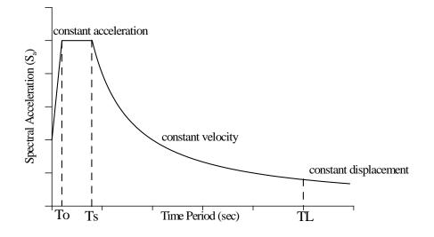
Figure 2: Typical Horizontal Elastic Design Spectrum.
