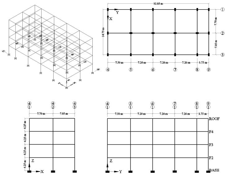
Figure 1: Three-Dimensional Computer Model and Geometry of the Building.
