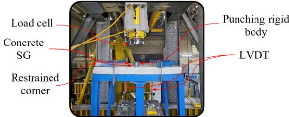
Figure (7): Test Scheme
