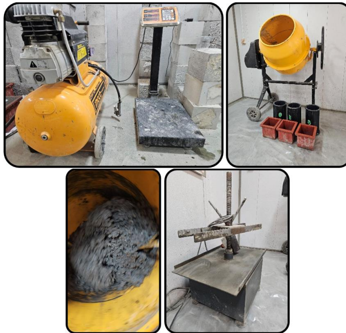
Figure (2): Instrumentations and tools for mixture design preparation
