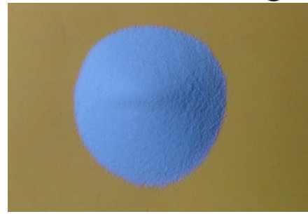
Figure (3): Aluminum Oxide (Al 2 O 3 ) powder The investigation of (Al 2 O 3 ) purity used in this study was conducted through the application of energy dispersive X-ray spectroscopy (EDX) using [the Bruker Company's XFlash_6110 model from Germany]. The findings are presented in Table (5), where it is worth noting that two elements (Au and Pt) were intentionally introduced into the material during the examination process. Subsequently, in Table (6), carbon was removed from the sample and through examination it became clear to us that the percentage of purity of the powder is (95.33805%).
