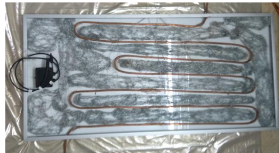
Figure (13): The method of applying a layer of stainless-steel swarf to the backside surface of the PV panel.
