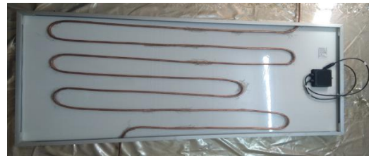
Figure (12): The route taken by the copper tube placed at the backside of the solar panel.
