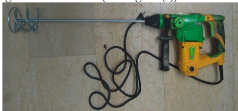
Figure (6): Electric mixing device
