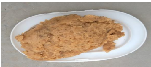
Figure (11): The Iraqi paraffin wax enriched with aluminum oxide ( Al_2O_3 )
