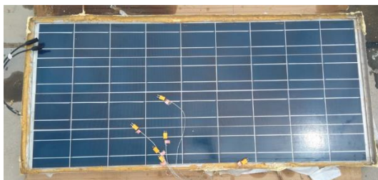
Figure (15): The final shape of the PV/T solar panel after modifications
