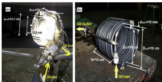
Figure 10. The dimensions of the cavity receivers utilized in the investigation are as follows: (a) cubical cavity; (b) cylindrical cavity [66].
