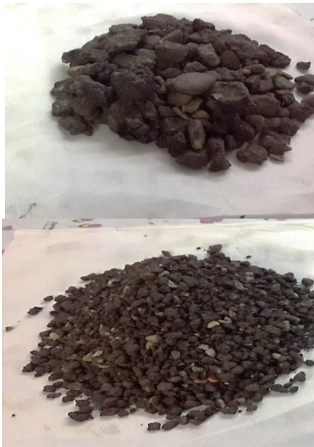
Figure (4): Samples of fractionated Reclaimed Asphalt Pavement (RAP) (coarse and fine).
