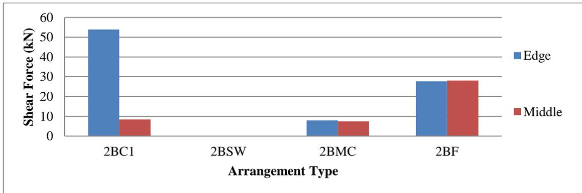
Figure 5: Shear force (kN) computed in the ground story for the two-bay building.
