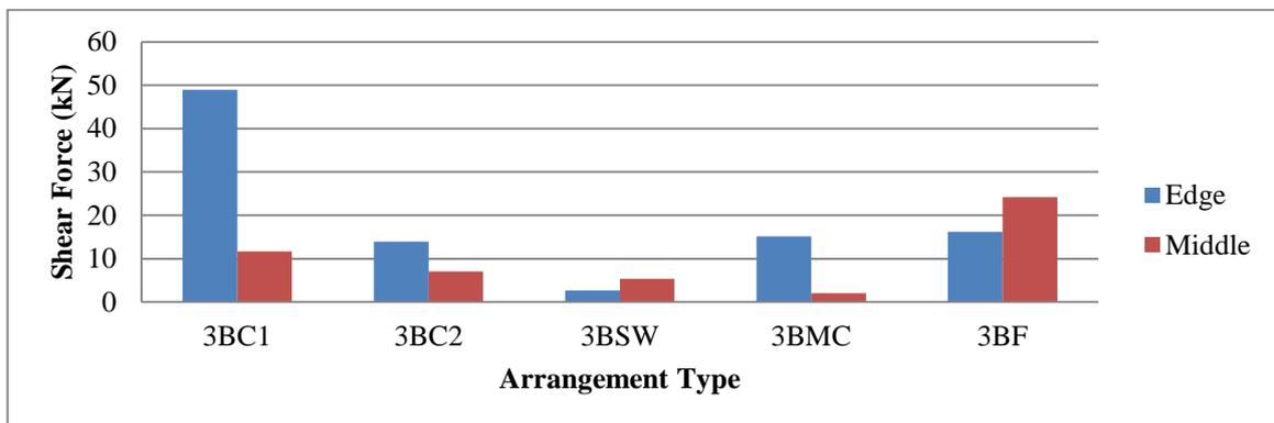
Figure 6: Shear force (kN) computed in the ground story for the Three-bay building.
