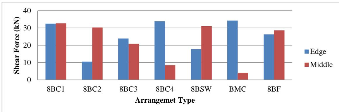
Figure 11: Shear force (kN) computed in the ground story for the eight-bay building.
