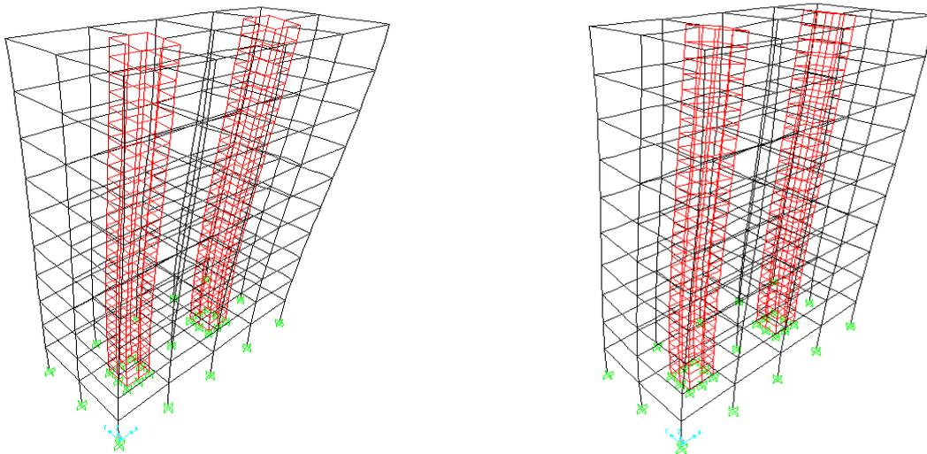
**Figure 3:** Mode shapes for a typical building (model 4BDC2).
