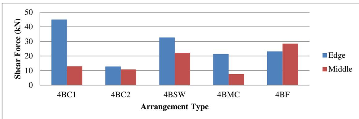
Figure 7: Shear force (kN) computed in the ground story for the Four-bay building.
