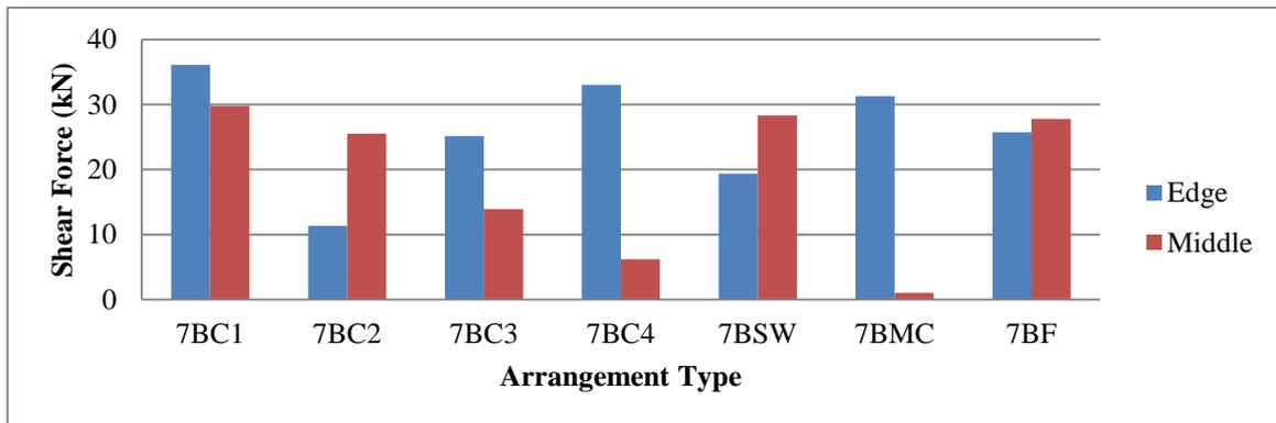
Figure 10: Shear force (kN) computed in the ground story for the seven-bay building.
