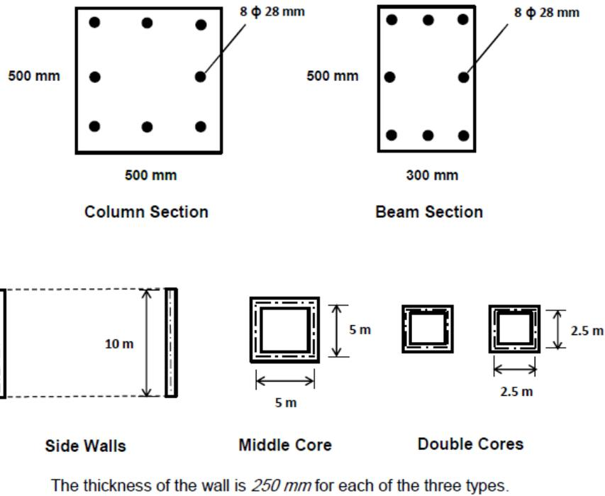
**Figure 2:** Details of sections of the members and dimensions of the shear walls.
