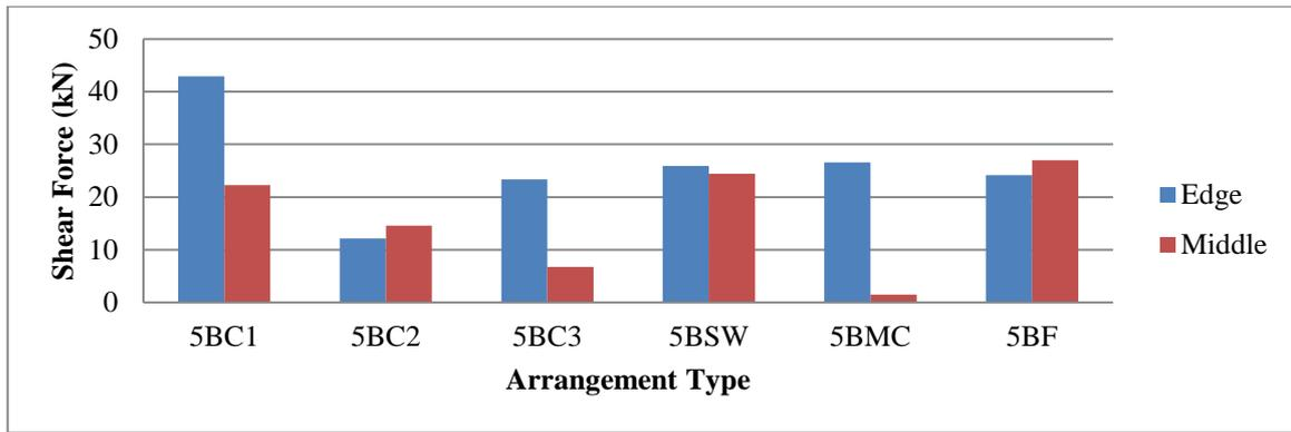
Figure 8: Shear force (kN) computed in the ground story for the Five-bay building.
