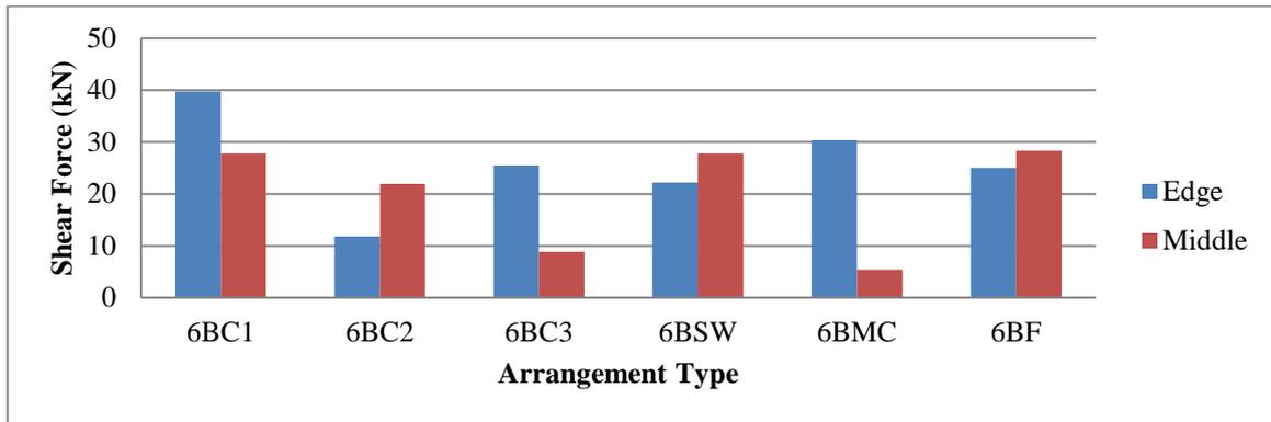
Figure 9: Shear force (kN) computed in the ground story for the six-bay building.
