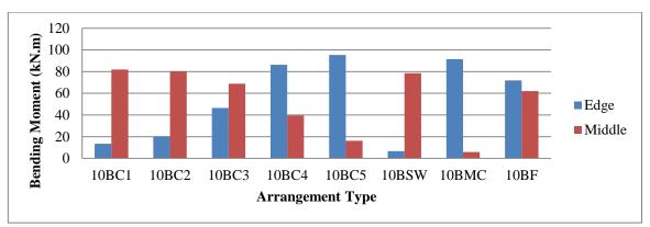
Figure 22: Bending moment (kN.m) computed in the ground story for the ten-bay building.
