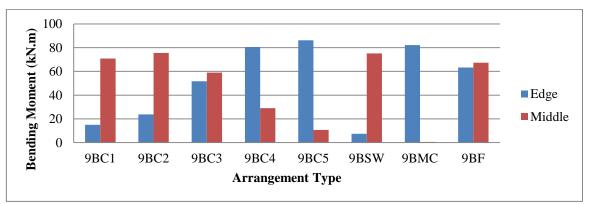
Figure 21: Bending moment (kN.m) computed in the ground story for the nine-bay building.
