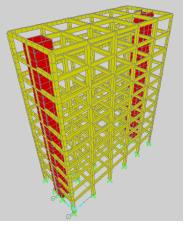
**Figure (1-f):** Double-core (C1) arrangement.
