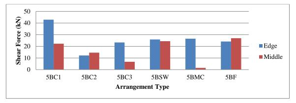
Figure 8: Shear force (kN) computed in the ground story for the Five-bay building.
