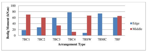
Figure 19: Bending moment (kN.m) computed in the ground story for the seven-bay building.
