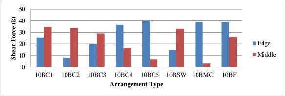
Figure 13: Shear force (kN) computed in the ground story for the ten-bay building.
