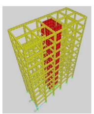
**Figure (1-c):** Middle-core arrangement.
