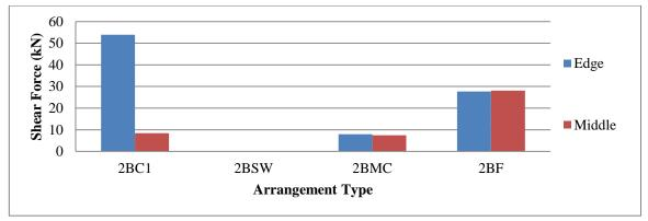
Figure 5: Shear force (kN) computed in the ground story for the two-bay building.
