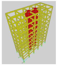
**Figure (1-d):** Double-core (C3) arrangement.
