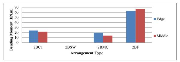
Figure 14: Bending moment (kN.m) computed in the ground story for the two-bay building.
