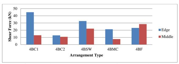
Figure 6: Shear force (kN) computed in the ground story for the Three-bay building.
