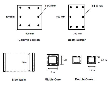
The thickness of the wall is 250 mm for each of the three types.
