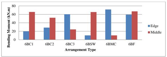
Figure 18: Bending moment (kN.m) computed in the ground story for the six-bay building.
