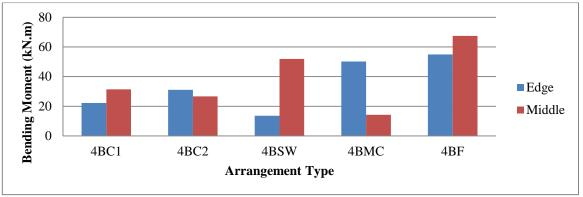
Figure 16: Bending moment (kN.m) computed in the ground story for the four-bay building.
