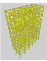
**Figure (1-a):** Free-wall arrangement.
