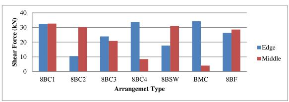
Figure 11: Shear force (kN) computed in the ground story for the eight-bay building.
