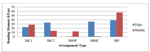
Figure 15: Bending moment (kN.m) computed in the ground story for the three-bay building.
