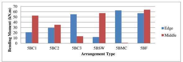
Figure 17: Bending moment (kN.m) computed in the ground story for the five-bay building.
