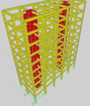
**Figure (1-e):** Double-core (C2) arrangement.
