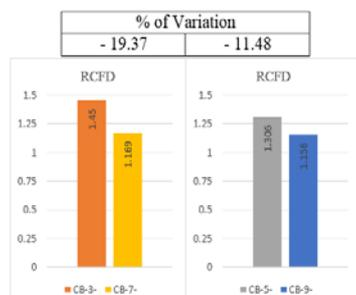
Figure (19): Effects of the shear connectors' intensity (i.e. number or spacing of stud shear connectors) on the residual cyclic flexural ductility for the composite beams subjected to displacement controlled non-reversible repeated loading.
