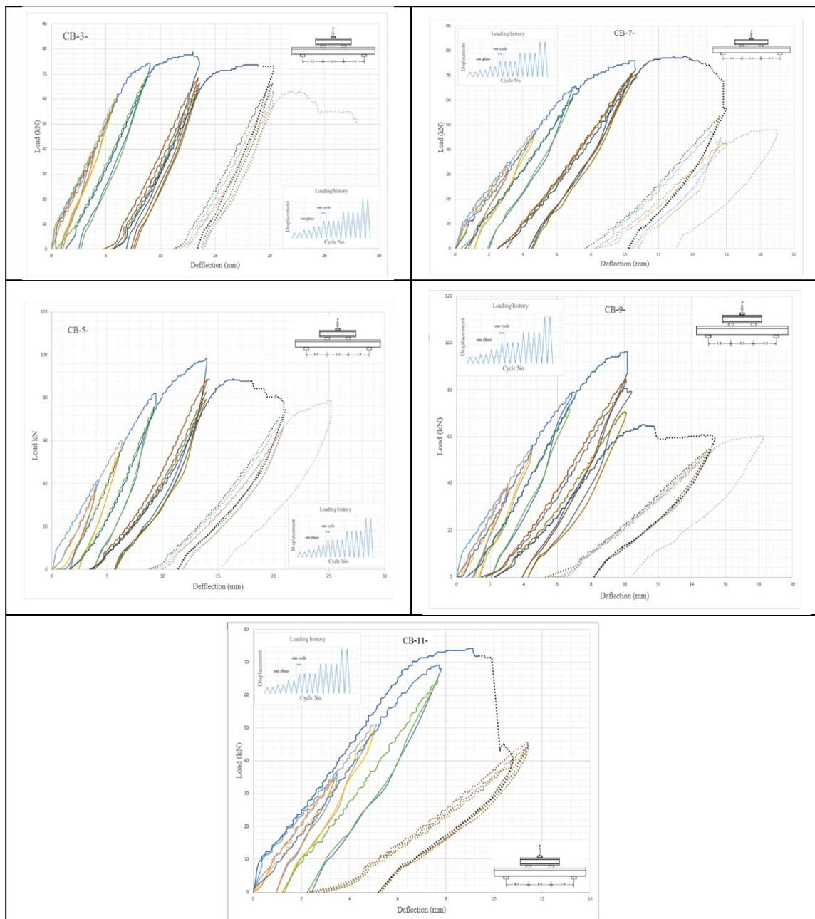
**Figure 9:** Load versus vertical deflection beneath the load responses till for the composite beams loaded by irreversible periodic repeated load as per attached loading history.
