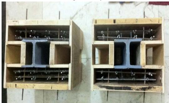
Plate 1: Push-out segments molds.
