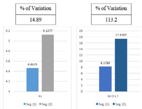
Figure (11): Effect of the shank length of the headed stud on its shear stiffness in push-out test
