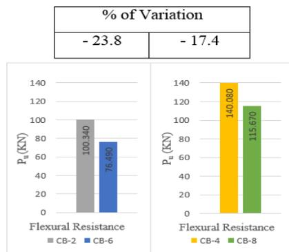
Figure (14): Effect of the shear-connection intensity (i.e. number or spacing of stud shear connectors) on the flexural resistance (represented by ultimate load capacity  $P_u$ ) for the monotonously loaded test composite beams.
