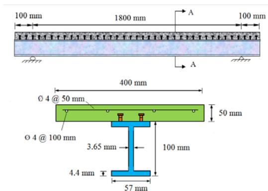
Figure 1: Typical simply supported beam layout (All dimension in mm).
