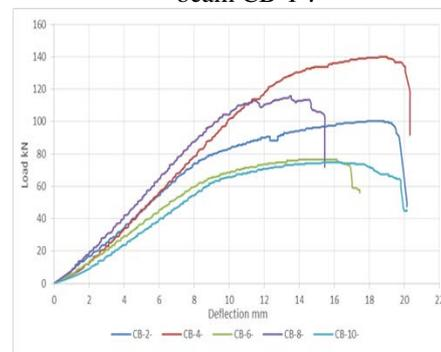
Figure 6: Load versus deflection relation for the monotonously loaded composite beam CB-2-, CB-4-, CB-6-, CB-8-, CB-10- respectively.
