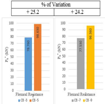
Figure (15): Effect of the proportions of the cross-section (dependent on strengthening by bottom steel) on the flexural resistance (represented by ultimate load capacity  $P_u^*$ ) for the composite beams subjected to displacement controlled non-reversible repeated loading.
