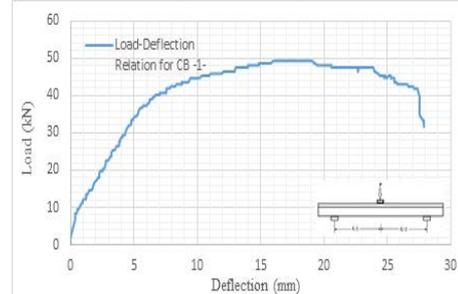
Figure 5: Load versus midspan deflection relation for the monotonously loaded composite beam CB-1-.
