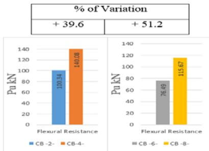
Figure (13): Effects of the proportions of the cross-section (dependent on strengthening by bottom steel plate) on the flexural resistance (represented by the ultimate load capacity  $P_u$ ) for the monotonously loaded test composite beams
