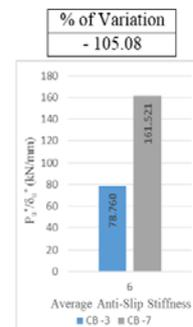
Figure (20): Effects of the shear-connectors intensity (i.e. number or spacing of stud shear connectors) on the average anti-slip stiffness  $P_{avg}/\delta_{avg}$  for the beams subjected to displacement non-reversible repeated loading.
