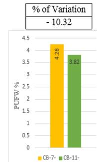
Figure (18): Effect of the overall length of the headed stud shear connectors on the percentage of post-ultimate flexural weakening (PUFW), for the composite beams subjected to displacement controlled non-reversible repeated loading.
