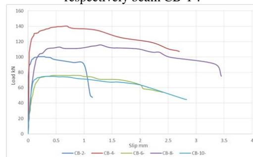
Figure 8: Load versus relative end slip relation for the monotonously loaded composite
