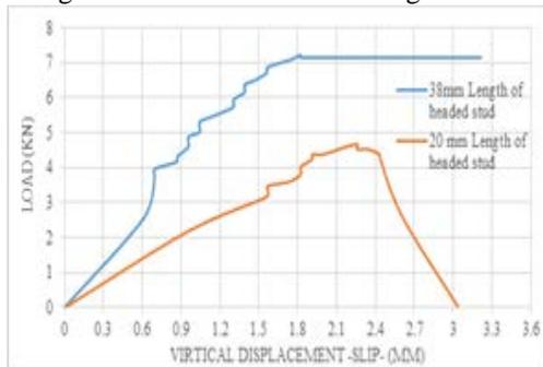
Figure 4: Load-slip relation for the segments.
