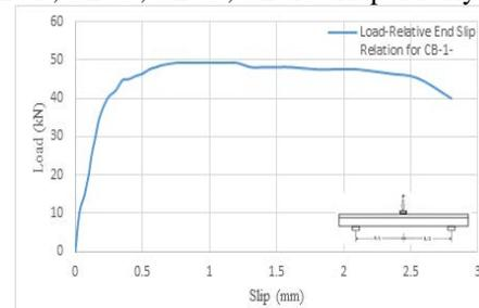
Figure 7: Load versus relative end slip relation for the monotonously loaded composite beam CB-2-, CB-4-, CB-6-, CB-8-, CB-10- respectively beam CB-1-.
