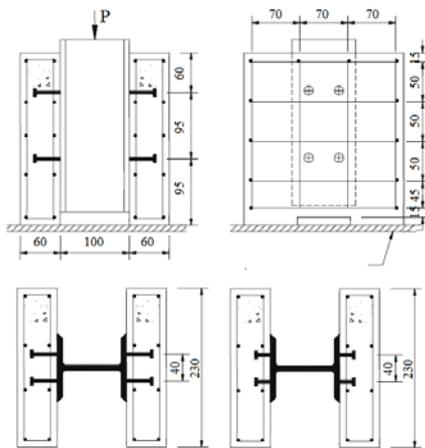
Figure 2: Push-out segments arrangements and geometry.
