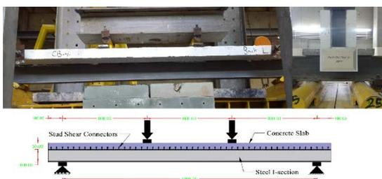
Plate 2: Typical test of composite beam and push-out segments.
