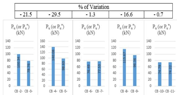
Figure (16): Effect of the type of load (monotonous or repeated) on the flexural resistance [represented by ultimate load capacity  $P_u$  or  $P_u^*$ ] for the test composite beams.
