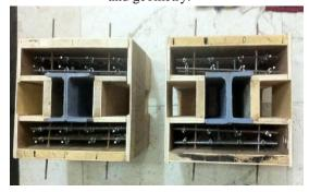
Plate 1: Push-out segments molds.
