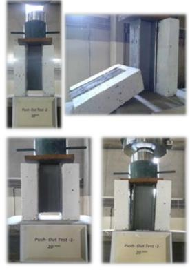
**Plate 3:** The first and the second push-out segments (of 20 mm and 38 mm length headed studs) subject to the standard test. (a) at of load application (b) at failure.
