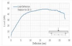
Figure 5: Load versus midspan deflection relation for the monotonously loaded composite
