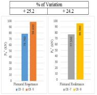
Figure (15): Effect of the proportions of the cross-section (dependent on strengthening by bottom steel) on the flexural resistance (represented by ultimate load capacity Pu<sup>\*</sup>) for the composite beams subjected to displacement controlled non-reversible repeated loading.
