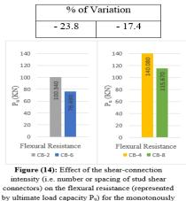
loaded test composite beams.
