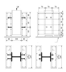
Figure 2: Push-out segments arrangements and geometry.
