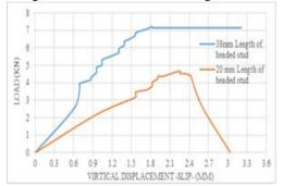
Figure 4: Load-slip relation for the segments.
