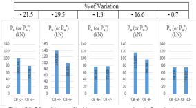
Figure (16): Effect of the type of load (monotonous or repeated) on the flexural resistance [represented by ultimate load capacity  $P_u$  or  $P_u^*$ ] for the test composite beams.
