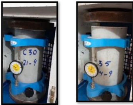
Figure (4): Elastic Modulus of Concrete.
