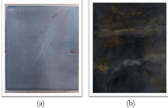
Figure (8): The pictures camera photos of carbon steel (a. before corrosion b. after 3h in NiCl 2 at 30°C)
