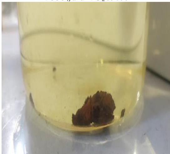
Figure (12): Beaker bottom at the end of the experiment at 30 °C and 1000 ppm \text{CuCl}_2 \cdot 2\text{H}_2\text{O} , for 100 rpm.
