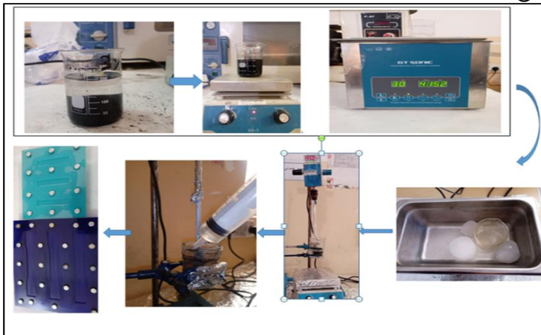
Figure (2): The processing steps of nanocomposites fabricating.
