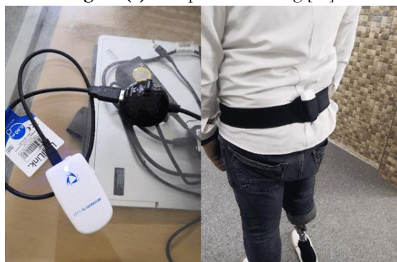
Figure (6): The amputee wears the G-Walk sensor and start the test.
