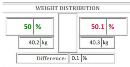
Figure (10): The weight distribution of the new prosthetic foot.
