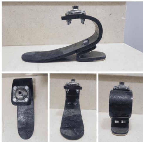
Figure (1): The carbon fiber prosthetic foot.
