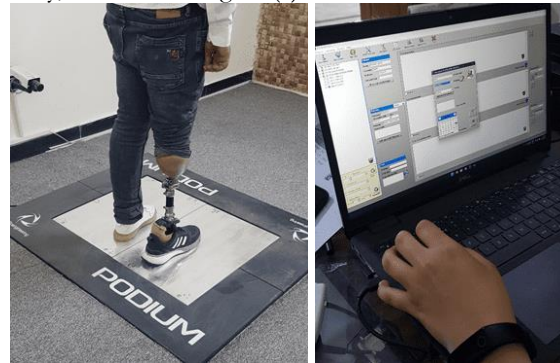
Figure (3): The amputee stands on the platform to begin testing protocols which include standing and walking in place.
