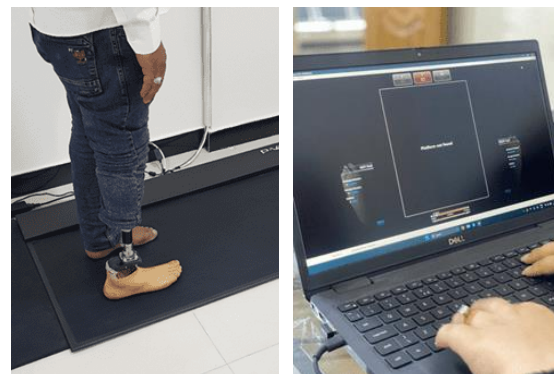
Figure (4): The amputee stands on the platform to begin testing protocols which include standing and walking in place.
