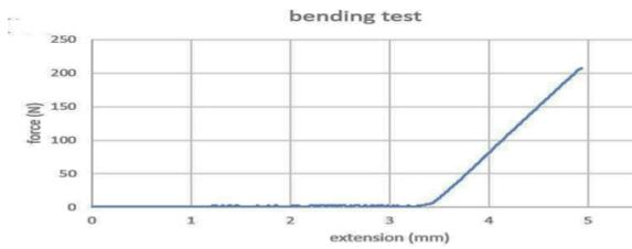
Figure (12): The stiffness curve (97%PMMA +3% HAp) for bending test
