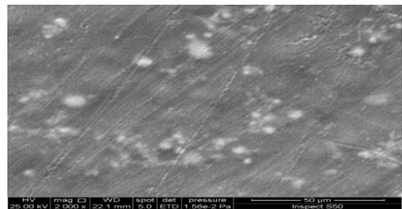
Figure (15): SEM image (97%PMMA +3% HAp) (The image is magnification 2000 X by using a voltage of 2500 kV and Everhart–Thornley detector (E–T detector or ET detector))
