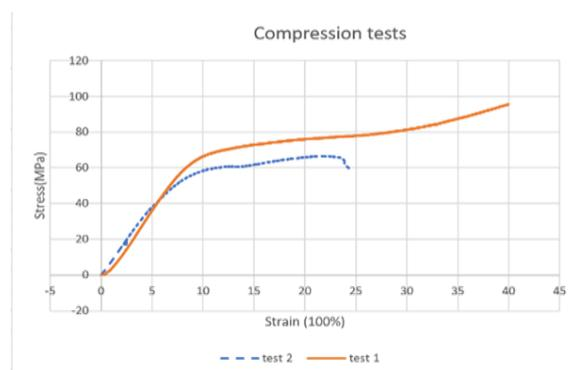
**Figure (11):** Stress-strain curve (97%PMMA +3% HAp) of compression test
