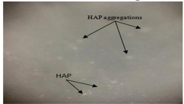
Figure (14): Optical microscopy image (97%PMMA +3% HAp)
