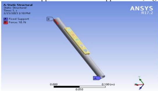
**Figure (8):** Boundary conditions in axial load (10N)
