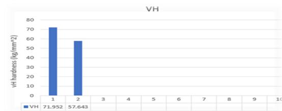
Figure (13): Results 97%PMMA +3% HAp) of Hardness test
