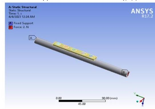
**Figure (9):** boundary conditions in bending load(2N)
