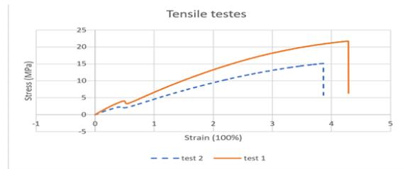
**Figure (10):** Stress-strain curve of the composite (97%PMMA +3% HAp)
