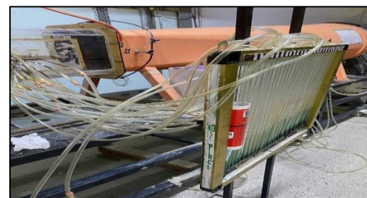
Figure (3): Setup of the Multi-tube Manometer for Measuring Surface Pressure Distribution
