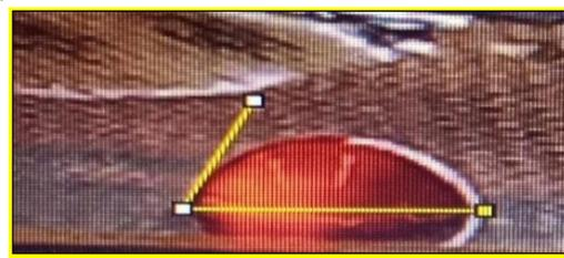
Figure (3): The specimen's dropping to measure the contact angle.
