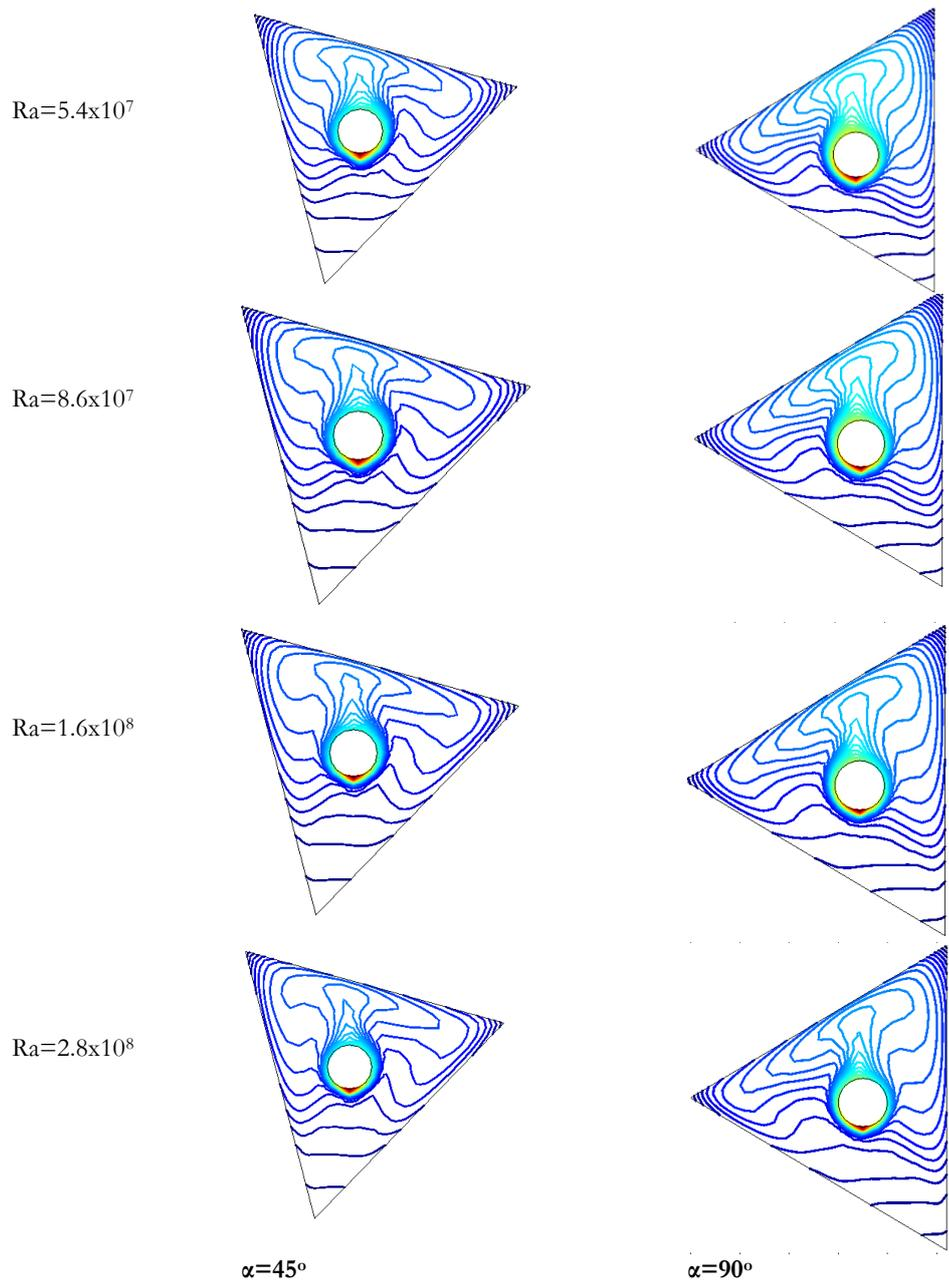
**Figure (6):** Isotherms contour at  $rr=0.345$ ,  $\alpha=45^\circ$  and  $90^\circ$  with different Rayleigh numbers.
