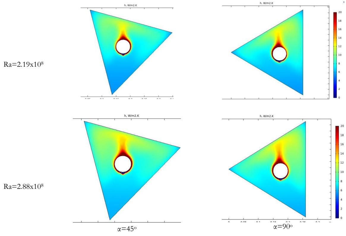
**Figure (9):** Isotherms contour at  $rr=0.345$ ,  $\alpha=0^\circ$ ,  $45^\circ$  and  $90^\circ$  with different Rayleigh numbers.
