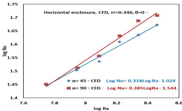
Figure (12): Logarithmic Nusselt number versus Logarithmic Rayleigh number for various  $\alpha$  at  $\theta=0^\circ$  and  $rr=0.35$ , CFD simulation.
