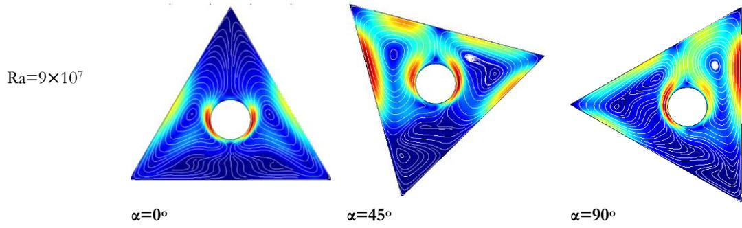
Figure (4): Stream lines contour at  $r=0.455$ ,  $\alpha=0^\circ$ ,  $45^\circ$  and  $90^\circ$  with different Rayleigh numbers
