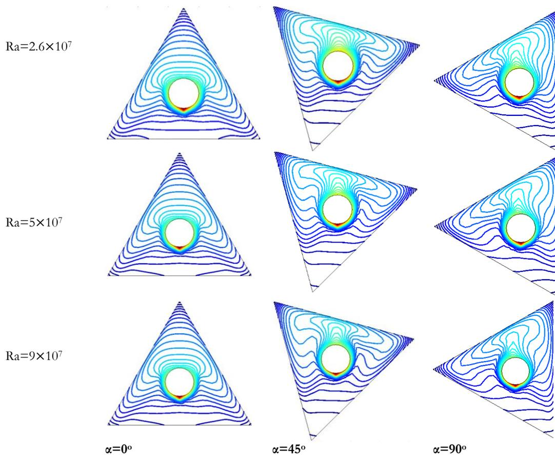
Figure( 7): Isotherms contour at  $rr=0.455$ ,  $\alpha=45^\circ$  and  $90^\circ$  with different Rayleigh numbers.
