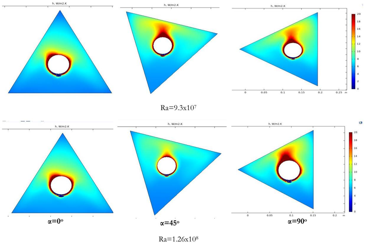
Figure (10): Isotherms contour at  $rr=0.455$ ,  $\alpha=0^\circ$ ,  $45^\circ$  and  $90^\circ$  with different Rayleigh numbers.
