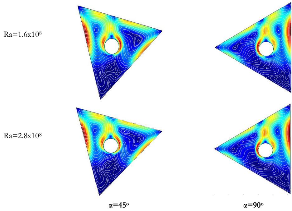
**Figure (3):** Stream lines contour at  $rr = 0.345$ ,  $\alpha = 45^\circ$  and  $90^\circ$  with different Rayleigh numbers.
