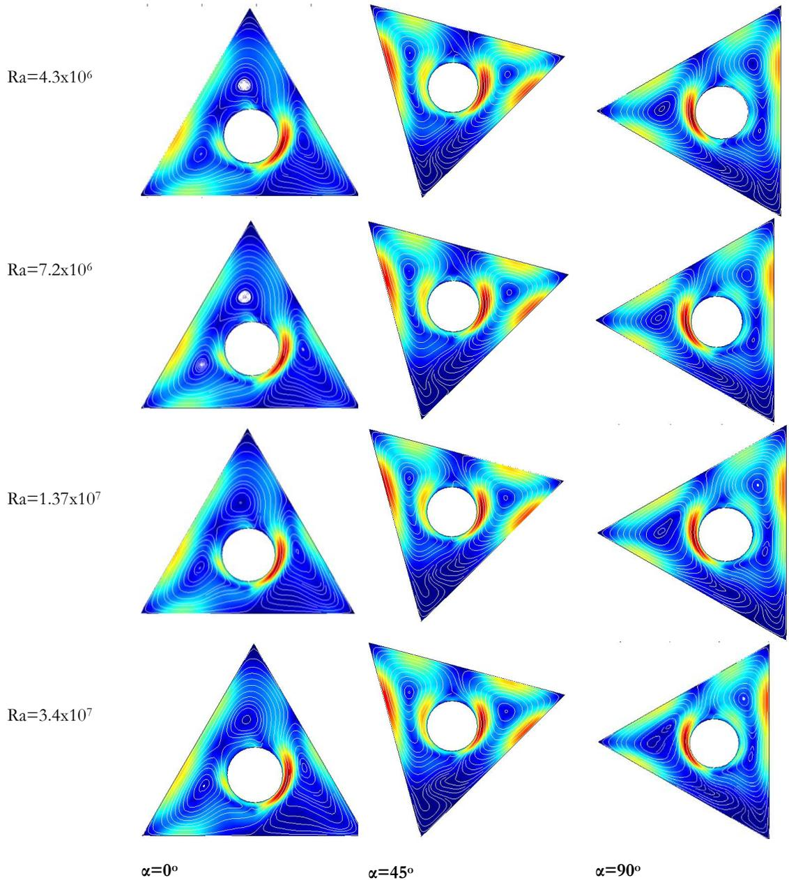
Figure (5): Stream lines contour at  $r = 0.618$ ,  $\alpha = 0^\circ$ ,  $45^\circ$  and  $90^\circ$  with different Rayleigh numbers.
