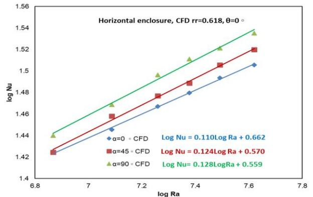
Figure (14): Logarithmic Nusselt number versus Logarithmic Rayleigh number for various  $\alpha$  at  $\theta=0^\circ$  and  $rr=0.618$ , CFD simulation.
