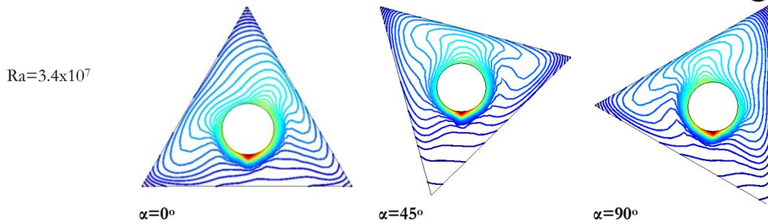
Figure (8): Isotherms contour at  $rr=0.618$ ,  $\alpha=45^\circ$  and  $90^\circ$  with different Rayleigh numbers.
