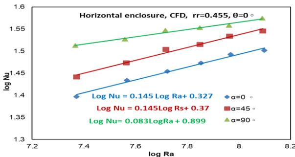
Figure (13): Logarithmic Nusselt number versus Logarithmic Rayleigh number for various  $\alpha$  at  $\theta=0^\circ$  and  $rr=0.455$ , CFD simulation.
